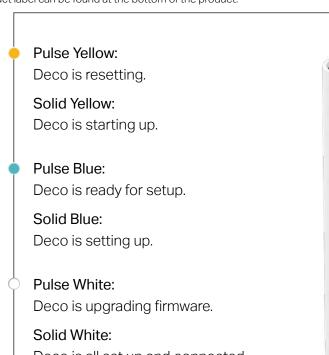
Deco is all set up and connected.
